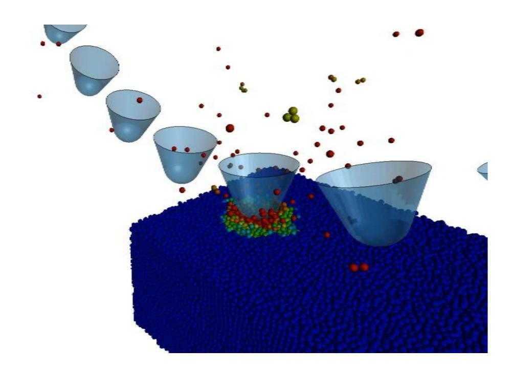
**Depth-of-cut 4 mm. Peak force varies** between 1.2 to 2.0 tons
